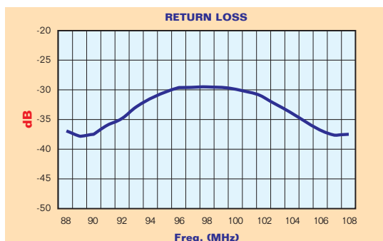
Typical return loss curve for splitter model DV/47/8-7/8
